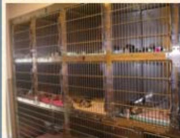
The photo above shows proper cages for cats in a shelter. The cages, food and water bowls, and litter boxes are all made of stainless steel, which is easy to clean with a bleach solution. The cages also do not open up to each other on the sides, and the fronts of the cages are at least 4 feet away from other cages, which helps decrease spread of pathogens.
